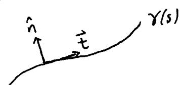
$$\begin{aligned} \hat{n} &= \left( -\frac{dy}{ds}, +\frac{dx}{ds} \right) = \text{normal} \\ \hat{t} &= \left( +\frac{dx}{ds}, +\frac{dy}{ds} \right) = \text{tangent} \\ \hat{n}^2 &= \hat{t}^2 = \left( \frac{dx}{ds} \right)^2 + \left( \frac{dy}{ds} \right)^2 = \frac{dx^2 + dy^2}{ds^2} = 1 \end{aligned}$$
