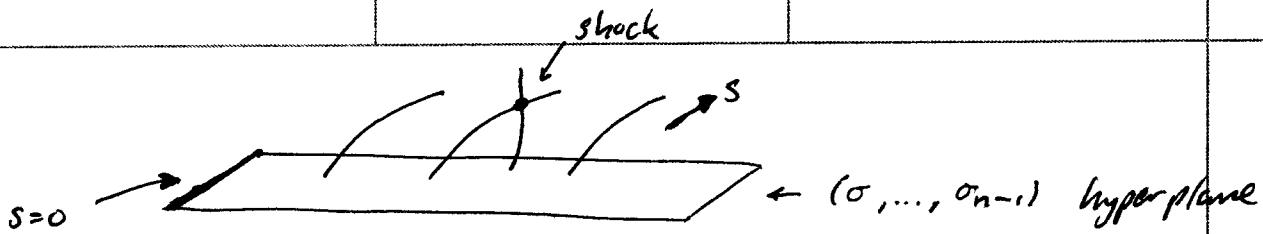
Characteristics are specified by  $\{\sigma_0, \dots, \sigma_{n-1}\}$ , and  $s$  is the (scaled) distance along the characteristic. When two characteristics cross, there is a shock.
