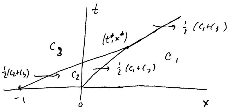
The trailing shock overtakes the leading shock at time  $t^*$ :
