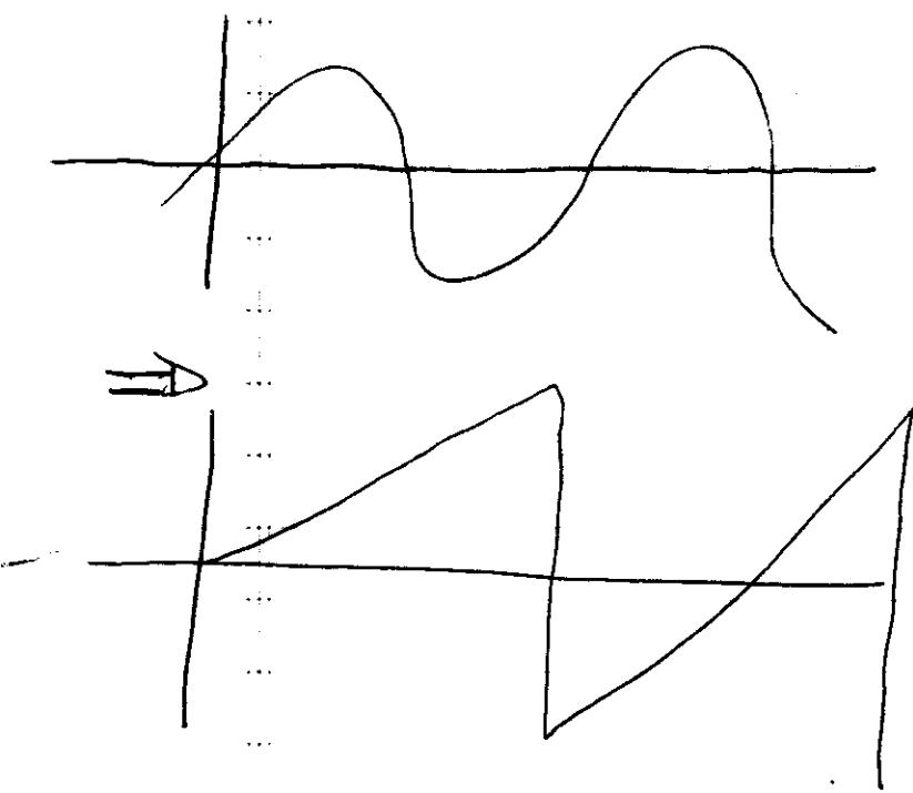
$$\left\{ \begin{array}{l} P = P_0 (\rho/\rho_0)^\gamma \\ C_s^2 = \frac{dP}{d\rho} = P_0 \gamma (\rho/\rho_0)^{\gamma-1} \\ C_s^2 \uparrow \text{with } \rho \end{array} \right.$$
