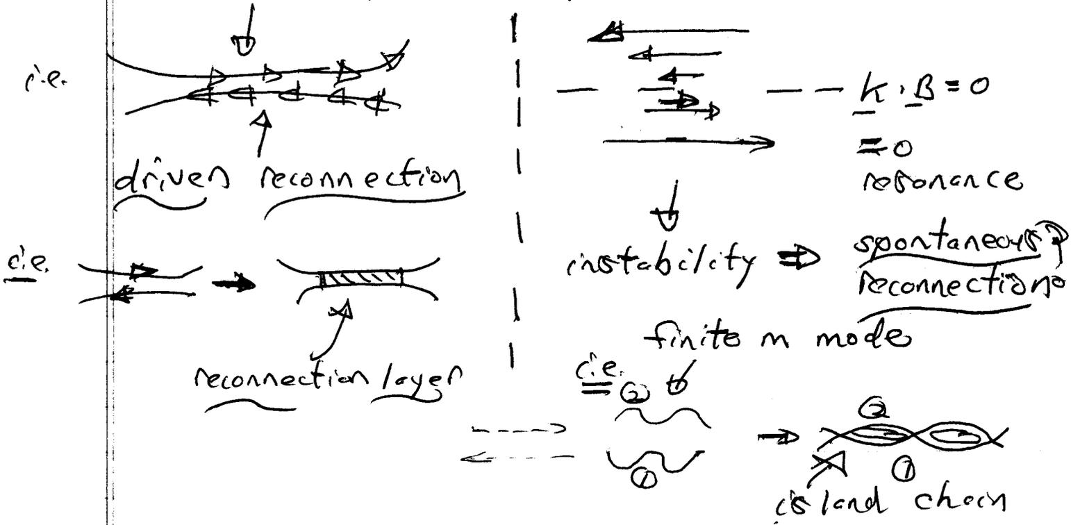
Note: - Resonant instability and  $\tilde{\psi}(x)$  ( $\tilde{B}_r(x)$ ) even parity in  $x$  ( $\tilde{\psi}(-x) = \tilde{\psi}(x)$ ), with  $\tilde{\psi}'(0) \neq 0 \Rightarrow$  "tearing"
