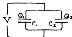
This is equivalent to two capacitors,  $C_1$  and  $C_2$  in parallel.
