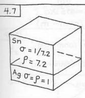
The ratio of conductivities, 7.2/1 and the ratio of layer thicknesses, 1/2, is all that matters. Let's take  $V_{Ag} = \int_{Ag} = 1$  and consider the cube that is 1/3 silver, 2/3 tin. For vertical currents the layers are in series and resistances add:
