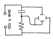
are equal, beam will trace elliptical pattern, in the sense indicated.
