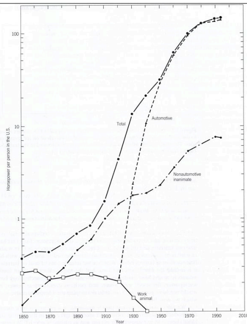
Figure 1.4 Horsepower per capita of all prime movers in the United States since 1850. Only a small fraction of this available horsepower is in use at any given time. (Source: Historical Statistics of the United States, Colonial Times to 1970 ; Statistical Abstracts of the United States 2003 , Washington, D.C.: U.S. Department of Commerce, Bureau of the Census.)
