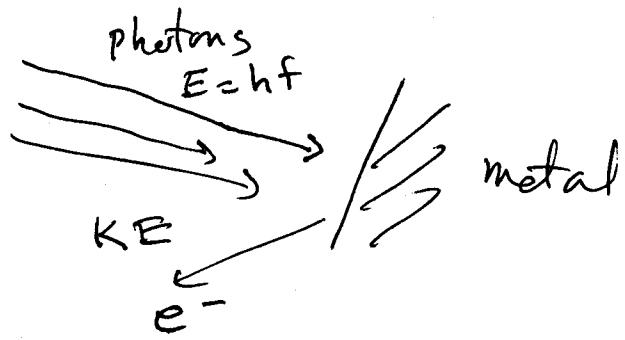
The stopping potential is a measure of the maximum kinetic energy of the photoelectrons produced by the light. The stopping potential is dependent on the frequency since this changes the photon energy. It is independent of the intensity since this does not change the photon energy. It only changes the no. of photons/sec.
