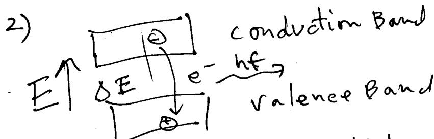
A semiconductor laser diode - the electron jumps from the conduction band to the valence band - the larger the band gap ΔE - the shorter the wavelength of the photon produced -
