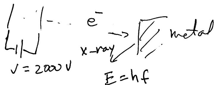
The shortest wavelength x-ray is produced when all the energy of the electron is transferred to the photon
