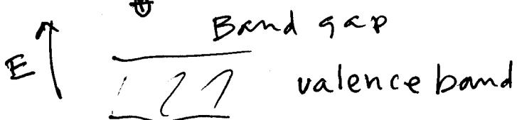
For an n-type semiconductor negative charge carriers are produced in the conduction band.
