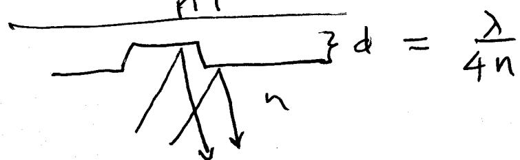
light hitting a pit interferes destructively with light hitting the outer surface to cause a decrease in intensity
