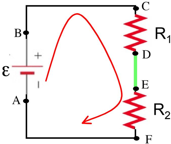
“The sum of voltage differences in going around a closed current loop is equal to zero”
