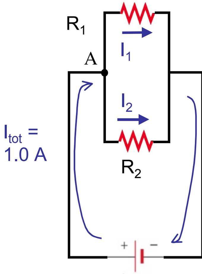
Suppose  $I_{\text{tot}} = 1.0 \text{ A}$ ,  $R_1 = 3 \Omega$  and  $R_2 = 6\Omega$ .
