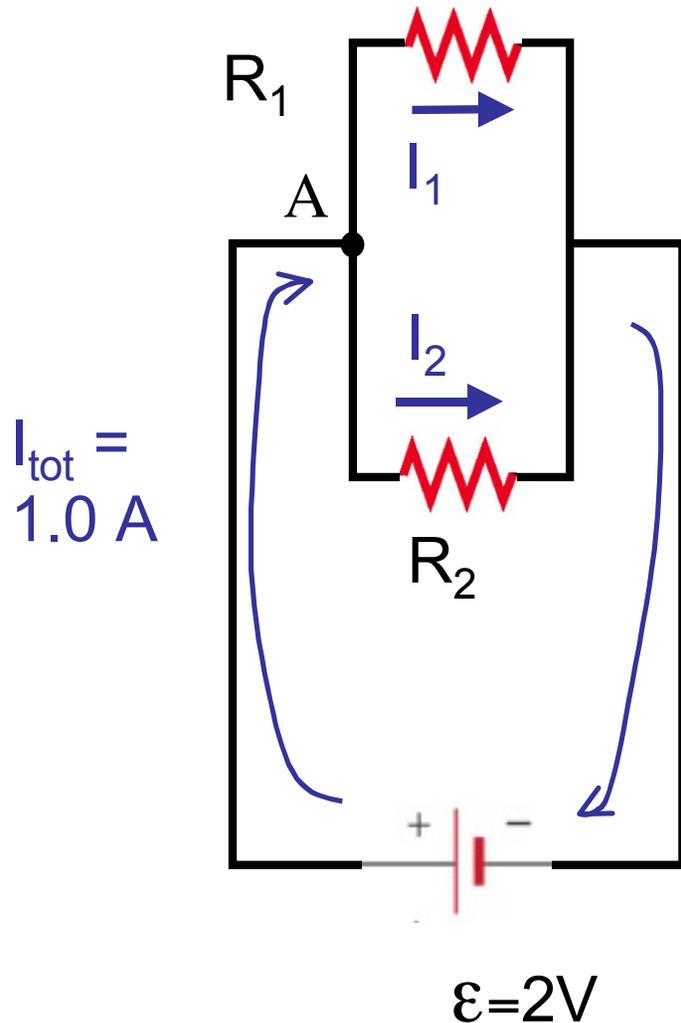
Confirm that the amount of the voltage drop across each resistor is 2V:
