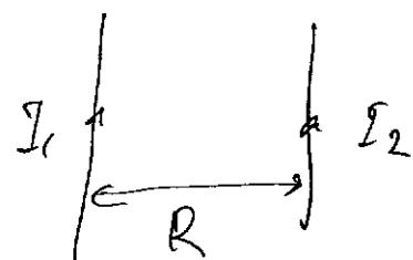
(a)  $B_1 = \frac{\mu_0 I_1}{2\pi R} = \underline{\underline{10^{-5} T \text{ (into the page)}}}$
