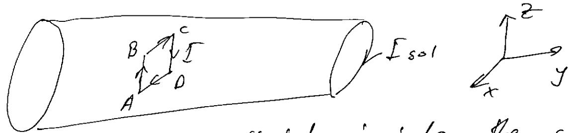
The magnetic field inside the solenoid points to the left and is equal to
