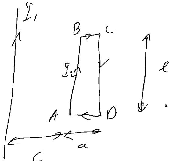
The field created by  $I_1$  at the location of the loop points into the page and is given by
