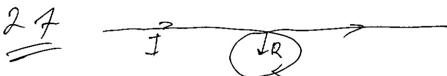
We have to add magnetic fields created by a long straight wire and a loop, at the center of the loop, both point into the page.
