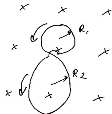
The induced EMF is as shown (by right hand rule). So the directions are opposite, the EMF in the bigger circle is bigger, so over all the direction of the induced current is:
