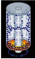
centrifugal separation gaseous UF_6
