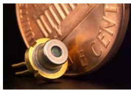
Laser diode Used in cd players etc.
