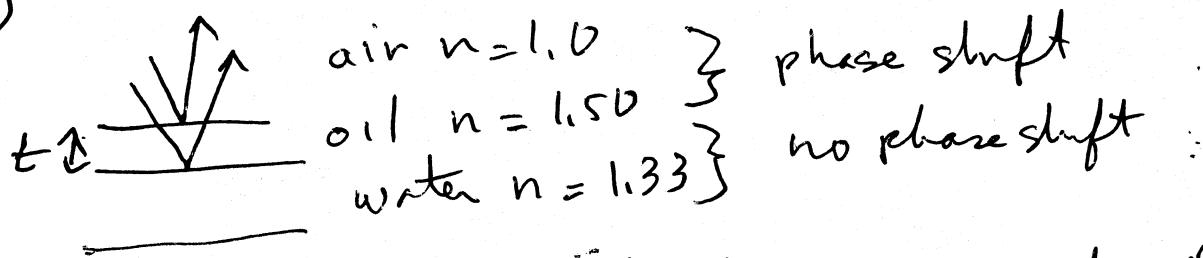
There is a phase shift difference of  $180^\circ$  between the two reflected waves. The condition for constructive interference is -
