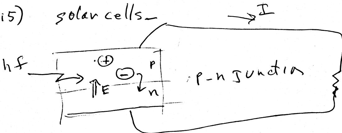
Electron-hole pairs are created by the absorption of a photon which are separated across the p-n junction giving a current
