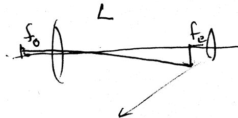
$$m = \frac{L}{f_o} \cdot \frac{25\text{ cm}}{f_e} = \frac{20\text{ cm}}{1.5\text{ cm}} \cdot \frac{25\text{ cm}}{3.0\text{ cm}} = 110$$
