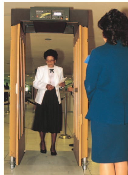
Figure 21.14 (Applying Physics 21.1) An airport metal detector.
