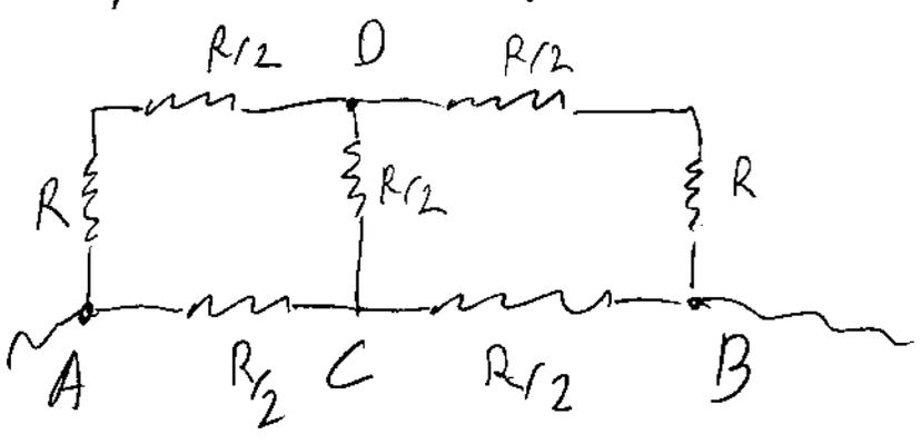
By symmetry, the current from A to C must be the same as the current from C to B, which means that there is no current from D to C, i.e. the resistance DC can be removed without changing anything.
