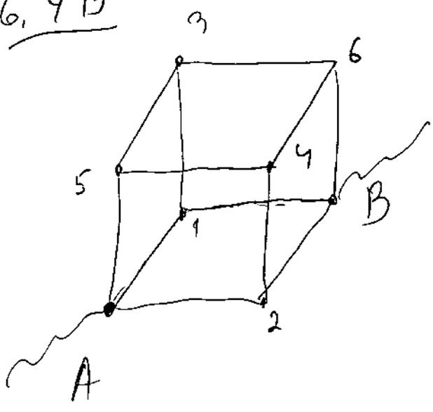
By symmetry, points 1 and 2 have the same potential, so they can be connected without changing the resistance. The same applies to points 3 and 4.
