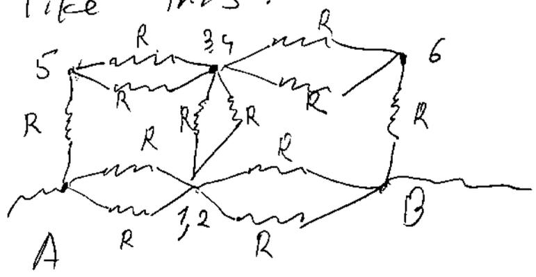
Then pairs of parallel R-s can be replaced by  $R/2$ :
