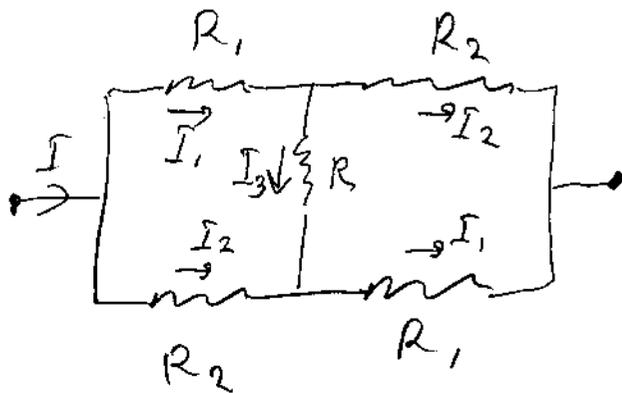
By symmetry, the current is the same through both  $R_1$ -s, also through both  $R_2$ -s, We have then
