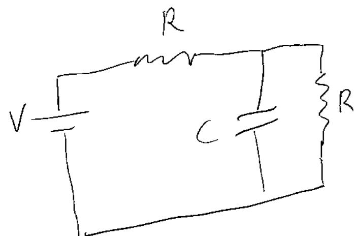
there is no current flowing to the capacitor and we have two resistors in series with the same current,
