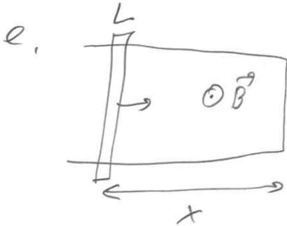
$$\begin{aligned} |\mathcal{E}| &= \frac{d\phi}{dt} = \frac{d(AB)}{dt} = \frac{d(BLx)}{dt} = \\ &= BL \frac{dx}{dt} = \underline{BLv} \end{aligned}$$
