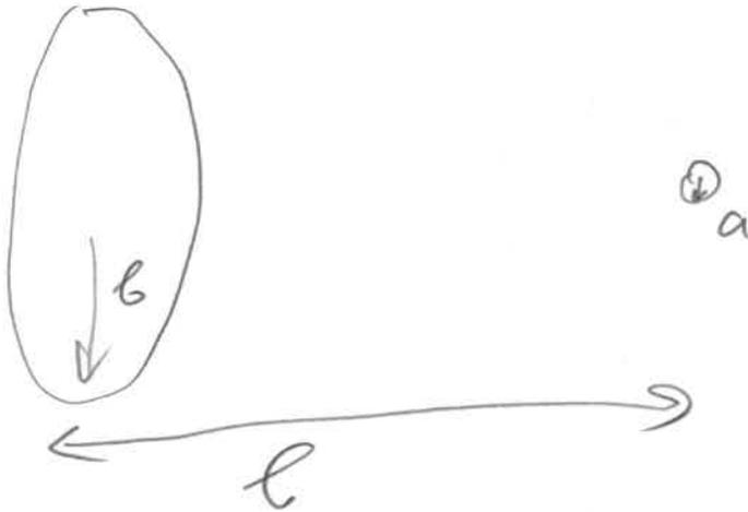
If  $b \gg a$  then the magnetic field through the small loop can be approximated by the value at the center. If there is current  $I$  through the big loop then
