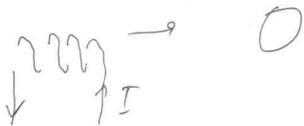
As view from solenoid the current in the loop will be opposite to that of the solenoid, i.e., clockwise.
