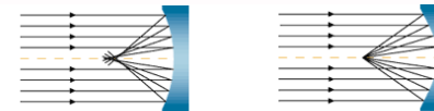
Spherical mirrors bring the light rays to different focal points, resulting in blurry images
