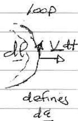
$$\frac{d\underline{a}}{dt} \cdot d\underline{a} = \underline{v} \cdot dt \times d\underline{l}$$
