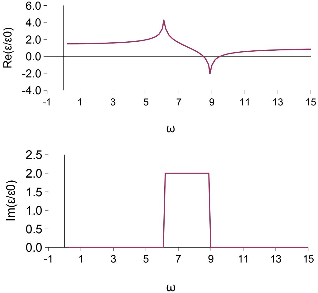
This looks quite similar to the results from the harmonic model. The difference is that the flat top of the imaginary part of the dielectric constant leads to an extended region of anomalous dispersion in the real part. Also the unrealistically steep walls of the imaginary part leads to infinite peaks in the real part.
