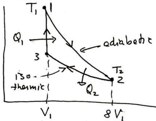
$Q_1$  = heat absorbed by gas during 3-1;  $Q_2$  = heat released by gas during 2-3
