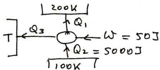
$$(a) Q_1 = 5049 \text{ J} \Rightarrow Q_3 = 1 \text{ J}, \text{ so } Q_2 + W = 5050 \text{ J} = Q_1 + Q_3$$
