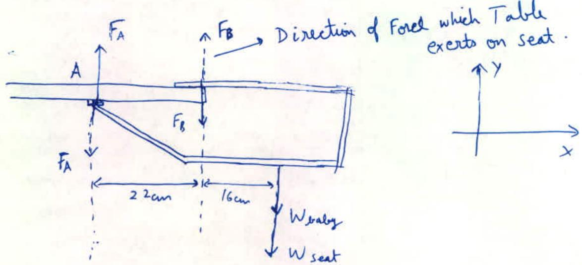
Balancing Torque about point A (where  $F_A$  is acting)
