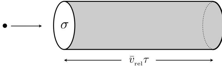
Figure 5.3: Graphic representation of the equation n \sigma \bar{v}_{\text{rel}} \tau = 1 , which yields the scattering time \tau in terms of the number density n , average particle pair relative velocity \bar{v}_{\text{rel}} , and two-particle total scattering cross section \sigma . The equation says that on average there must be one particle within the tube.
