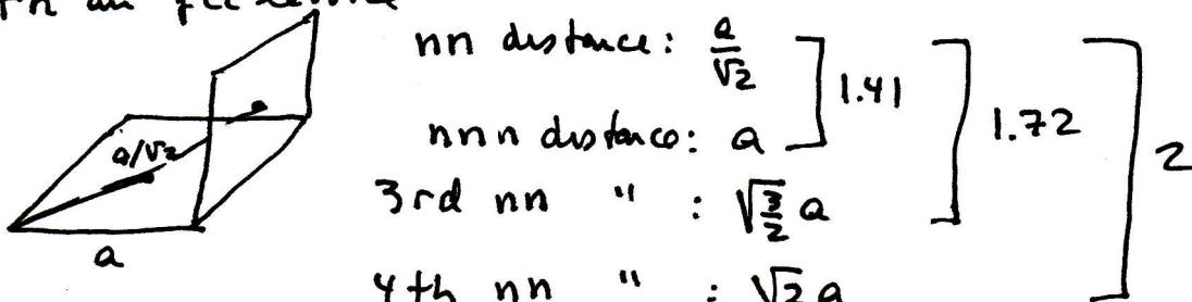
So B  $\Rightarrow$  an fcc reciprocal lattice  $\Rightarrow$  direct lattice  $\Rightarrow$  BCC fn B
