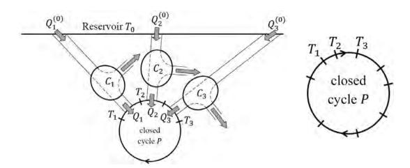
**Proof of Clausius's 's inequality.** For a derivation we divide the cycle  $P_c$  into n segments so that on each segment its temperature  $T_i$  (i = 1, ..., n) is constant.
