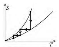
Note that all entropy curves converge to  $S(T \to 0) \to 0$ . The process becomes hence progressively ineffective and an infinite number of Linde iterations would be needed to reach the limit  $T \to 0$ .
