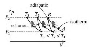
Using a gas as a working substance, cooling is achieved by the *Linde method* through a sequence isothermal and adiabatic transformations.
