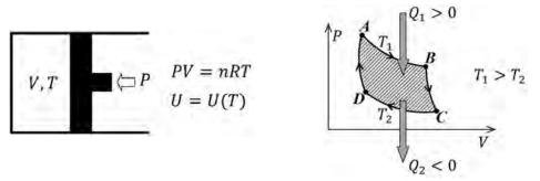
One Carnot cycle consists of four consecutive thermodynamic processes, which can be realized with an arbitrary working substance. We shall consider here however the case of an ideal gas.
