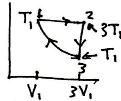
$$\Rightarrow \text{total net work in cycle: } W = RT_1(2 - \ln 3) = 0.90RT_1$$
