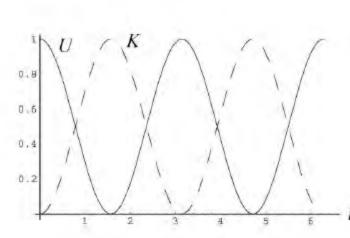
28. The total mechanical energy is equal to the (maximum) kinetic energy as it passes through the equilibrium position (x = 0):
