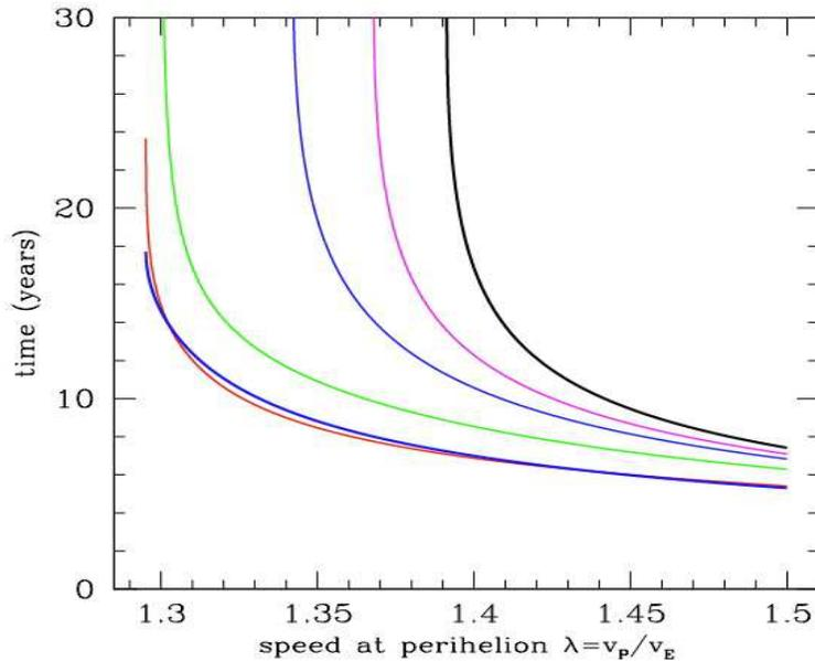
Figure 9.12: Total time for Earth-Neptune mission as a function of dimensionless velocity at perihelion,  $\lambda = v_p/v_E$ . Six different values of  $\kappa$ , the value of perijove in units of the Jovian radius, are shown:  $\kappa = 1.0$  (thick blue),  $\kappa = 5.0$  (red),  $\kappa = 20$  (green),  $\kappa = 50$  (blue),  $\kappa = 100$  (magenta), and  $\kappa = \infty$  (thick black).
