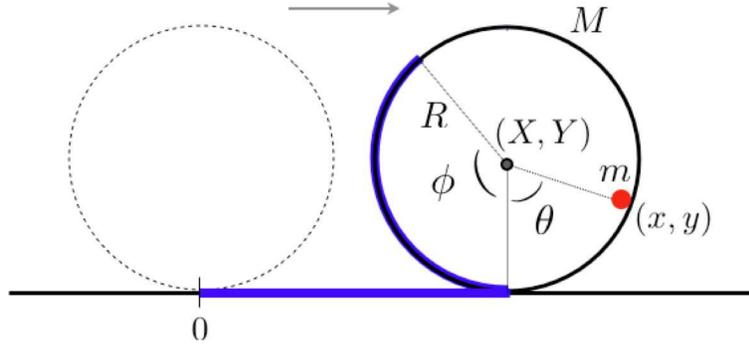
Figure 8.7: A point mass  $m$  inside a hoop of mass  $M$ , radius  $R$ , and moment of inertia  $I$ .
