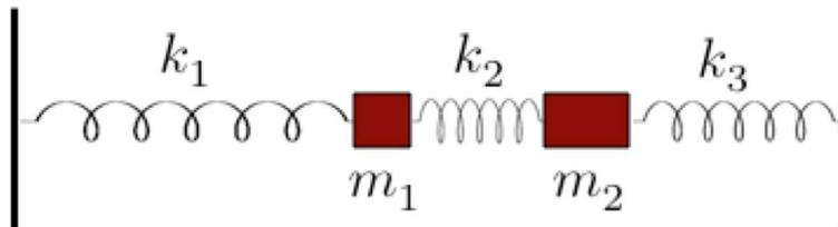
Figure 10.1: A system of masses and springs.
