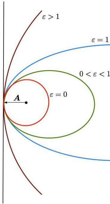
Figure 9.5: Keplerian orbits are conic sections, classified according to eccentricity: hyperbola ( $\epsilon > 1$ ), parabola ( $\epsilon = 1$ ), ellipse ( $0 < \epsilon < 1$ ), and circle ( $\epsilon = 0$ ). The Laplace-Runge-Lenz vector,  $\mathbf{A}$ , points toward periapsis.
