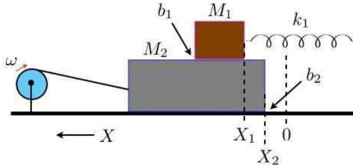
Figure 4.6: The equivalent mechanical circuit for fig. 4.5.
