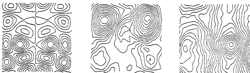
Figure 3. Contours of constant stream function corresponding to the situation shown in figure 1. The times corresponding to the three (instantaneous) sets of streamlines are the initial time, a time halfway through the run, and a time at the end of the run (from left to right).
