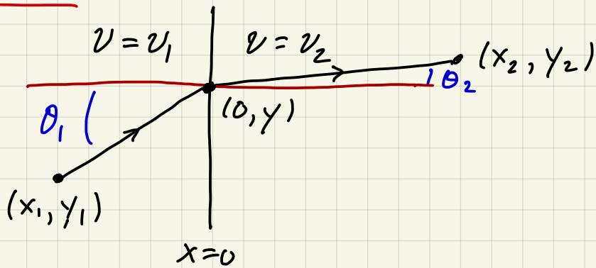
$$T(y) = \frac{1}{v_1} \sqrt{x_1^2 + (y - y_1)^2} + \frac{1}{v_2} \sqrt{x_2^2 + (y_2 - y)^2}$$
