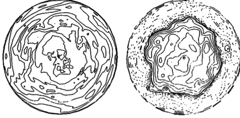
Figure 2. Equipotential contour of simulation results obtained from equations (21) and (22). The solid (dotted) lines are for positive (negative) equipotentials. It is clear that the curvature driven plasma turbulence produces a self-organized state in which a global equipotential has a \phi = 0 closed surface near the outer edge of the plasma.
